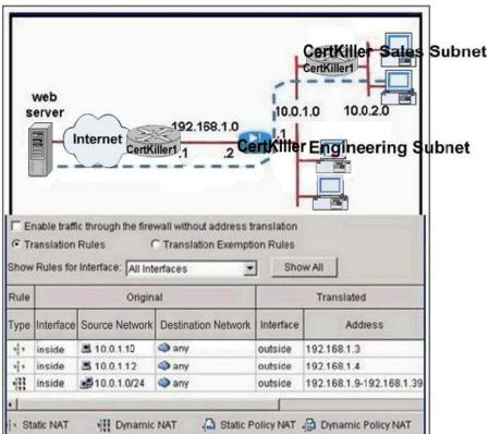
You work as a network technician at Certkiller .com. Host Certkiller A on the CertK in Sales subnet (10.0.2.0/24) is not able to initiate a web connection to an outside website. According to the network diagram and the partial Cisco Adaptive Security Device Manager configuration shown in the exhibit, what is the cause of the problem?
