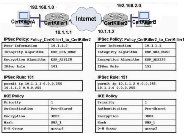
The tables contain information from the Cisco Router and Security Device Manager configuration of Router Certkiller 1 and Router Certkiller 1. Traffic between Host Certkiller A and Host Certkiller B is not successfully establishing the site-to-site VPN between Router Certkiller 1 and Router Certkiller 2. What is the mostly likely cause of this fault?
