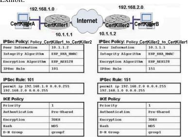
The tables contain information from the Cisco Router and Security Device Manager configuration of Router Certkiller 1 and Router Certkiller 2. Traffic between Host 1 and
