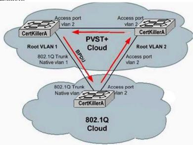
Switches A and C are running PVST+ STP, and Switch B is running 802.1Q STP. If the BPDU of the root in VLAN 1 is better than the BPDU of the root in VLAN 2, then there is no blocking port in the VLAN 2 topology. The BPDU of VLAN 2 never makes a "full circle" around the topology; it is replaced by the VLAN 1 BPDU on the B-C link, because B runs only one STP merged with VLAN 1 STP of PVST+. Thus, there is a forwarding loop. What does PVST+ do to correct this?
